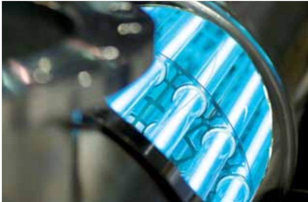
this, a constantly high UV light yield is achieved with a substantially extended lamp service life at the same time. Moreover, by using this technology, it is no longer necessary to apply liquid mercury inside the lamp.
