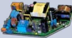
Electronic ballasts ensure that the Spektrotherm® UV lamps operate cost-effectively and reliably
